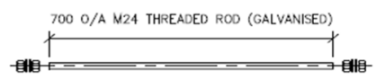
ENLARGED DETAIL OF M24 H.D. BOLT THREADED ROD TO BE SUPPLIED COMPLETE WITH 4-NUTS AND 4-WASHERS (SCALE 1:10)
